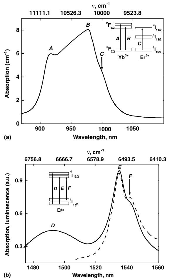
Fig. 1. Absorption (solid) and emission (dashed curves) spectra of the Er, Yb: boro-silico-phosphate-glass: (a) absorption spectrum in the spectral region of 870–1050 nm; (b) absorption and emission spectrum in the spectral region of 1475–1560 nm.
