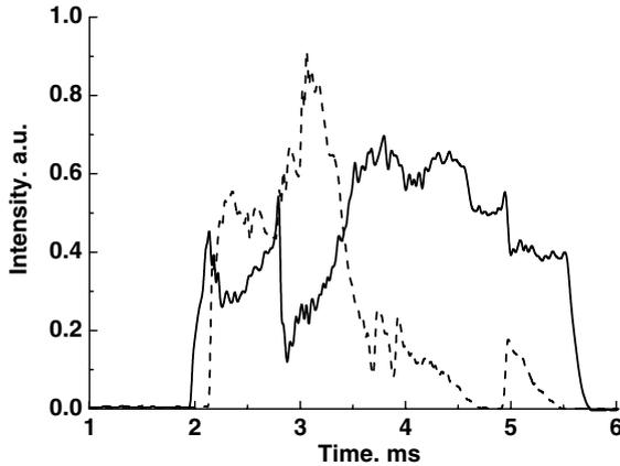
Fig. 4. Temporal profiles of the laser light pulses for 1533–1537 nm (solid) and 1541–1545 nm (dashed curves) spectral ranges averaged per 100 pulses for the free-running Er, Yb: glass laser operation at the pump power about 100 W.
