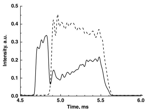
Fig. 3. Temporal profiles of the laser light pulses for 1533–1537 nm (solid) and 1541–1545 nm (dashed curves) spectral ranges averaged per 100 pulses for the free-running Er, Yb: glass laser operation at the pump power about 40 W.
