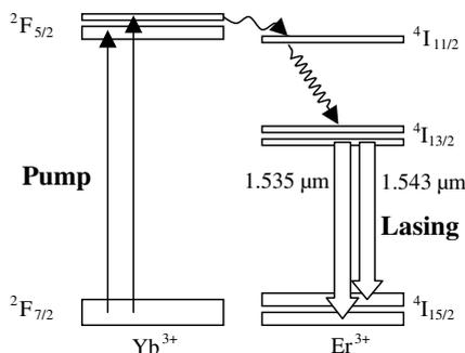
Fig. 5. Energy levels diagram and pumping scheme of Er, Yb: glass laser.
