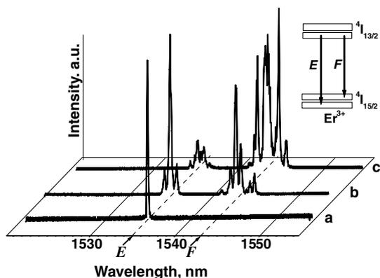
Fig. 2. Spectrum of lasing for the free-running Er, Yb: glass laser operation at the pump power of about 1–30, 2–60, 3–100 W.
