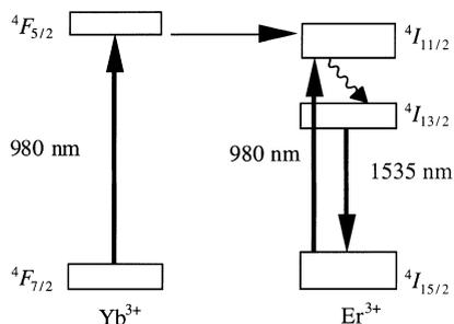
Fig. 1. Schematic representation of the levels involved in the optical processes. The solid line arrows indicate the absorption and emission transitions for the  $\text{Er}^{3+}$  and  $\text{Yb}^{3+}$  ions. The wavy lines represents the non-radiative decay  $^4I_{11/2} \rightarrow ^4I_{13/2}$  and the thin arrow stands for the energy transfer.
