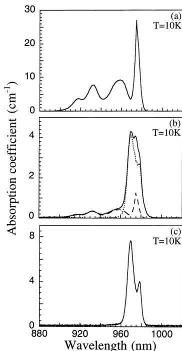
Fig. 6. Absorption spectra in the 980 nm band of sample A (a), sample B (b, solid line) and sample C (c). In (b) it is also shown the contribution of  $\text{Er}^{3+}$  to the absorption spectrum (dots), obtained by subtracting the  $\text{Yb}^{3+}$  absorption spectrum (dashed line).
