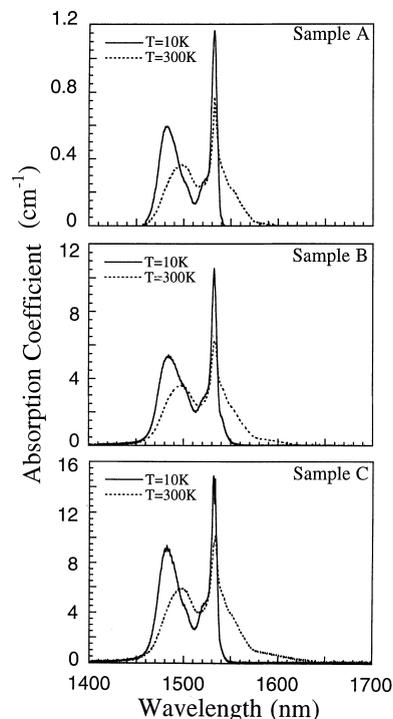
Fig. 2.  $\text{Er}^{3+} \ ^4I_{15/2} \rightarrow ^4I_{13/2}$  absorption spectra, measured at 10 K (solid lines) and room temperature (dashed lines), of the three samples.
