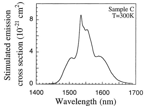
Fig. 5. Stimulated emission cross section of sample C at room temperature.
