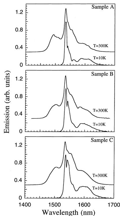
Fig. 4.  $\text{Er}^{3+}$   ${}^4\text{I}_{13/2} \rightarrow {}^4\text{I}_{15/2}$  emission spectra for the three samples at  $T=10\text{ K}$  and at room temperature.
