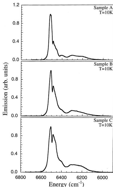
Fig. 3. Emission spectra measured at 10 K of the  $\text{Er}^{3+}$   ${}^4\text{I}_{13/2} \rightarrow {}^4\text{I}_{15/2}$  transition for the three samples.
