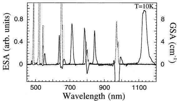
Fig. 7. Excited State Absorption (ESA, solid line) and Ground State Absorption (GSA, dashed line) spectra of sample C at 10 K.
