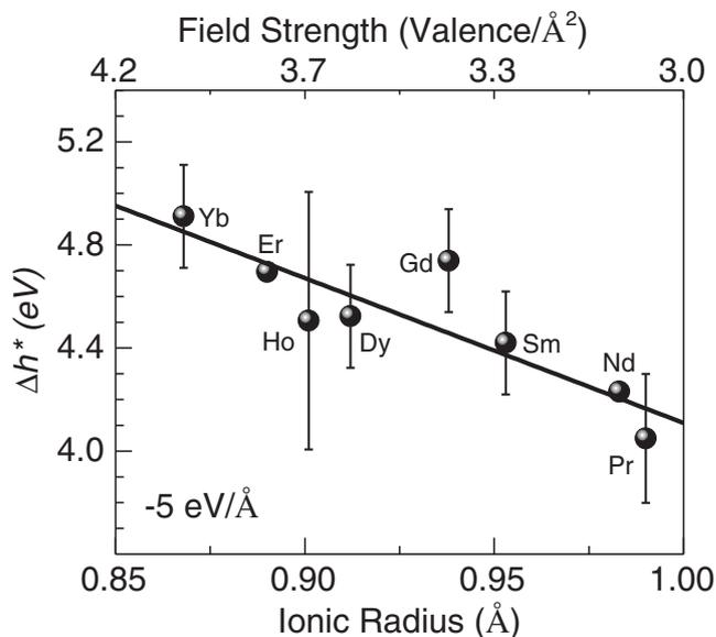
**Fig. 4.** Glass transition activation energy vs. the RE ionic radius [12] (bottom scale) and the field strength (top scale).
