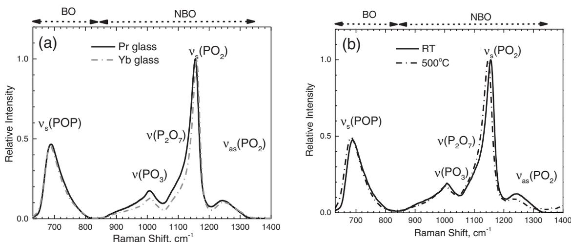
**Fig. 5.** Normalized Raman spectra and mode assignments for (a) the two extreme compositions, Yb and Pr glass and (b) Pr glass at room temperature (RT) and at 500 °C.
