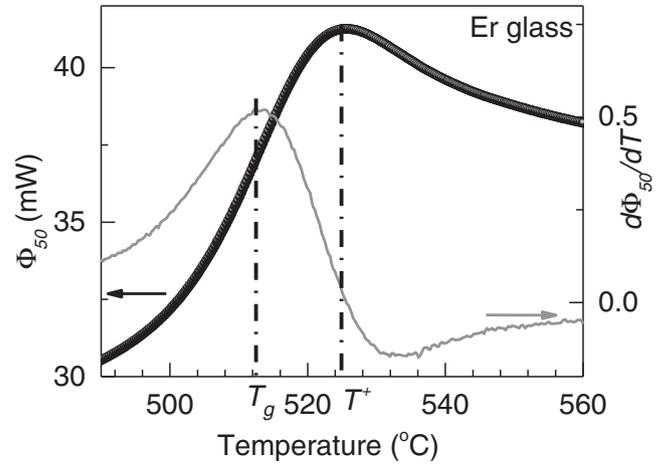
Fig. 2. Example for  $T_g$  assessment at the point of maximum slope of the heat flow curve  $\Phi_{50}(T)$  for Er glass. The grey trace is the first derivative of the heat flow. The heating rate of 50 °C/min is indicated by the subscript.
