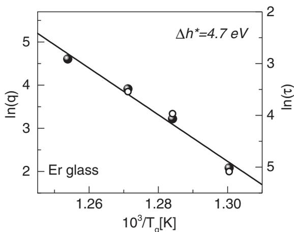
**Fig. 3.** Arrhenius-like plot for Er glass:  $q$  (left axis, solid symbols) is the heating rate in °C/min;  $\tau$  (right axis, open symbols) is the relaxation time in seconds.
