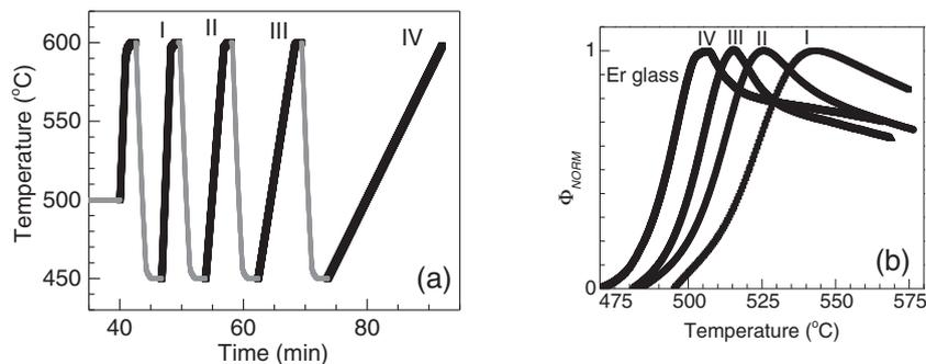
Fig. 1. (a) Thermal cycling procedure for all samples. Only the Pr glass was annealed at 450 °C. Data for the following heating segments were analyzed: I.  $q = 100$  °C/min; II.  $q = 50$  °C/min; III.  $q = 25$  °C/min; IV.  $q = 8$  °C/min. (b) Normalized heat flow data ( $\Phi_{\text{NORM}}$ ) for the Er glass corresponding to the thermal cycling procedure in (a).
