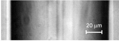
Fig. 1. Third-order 1.59- $\mu\text{m}$  pitched FBG made with IR femtosecond radiation in the core and cladding of the phosphate glass fiber.
