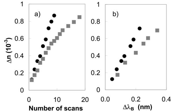
Fig. 3. Growth dynamics of  $\Delta n$  versus (a) number of sweeps of the laser beam and (b) the wavelength shift  $\Delta\lambda_B$  of the phosphate grating (black dots) and silica grating (gray squares) under the same writing conditions (1000  $\mu\text{J}/\text{pulse}$ , 50 Hz).
