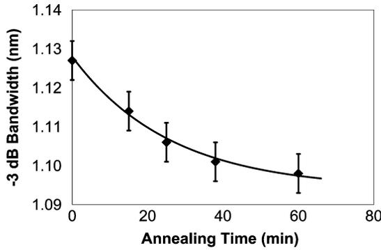
Fig. 4. Isothermal decay of the phosphate refractive index variation at 300 °C follows an exponential decay (solid line). The 5-pm error in the bandwidth measurement is denoted by error bars.
