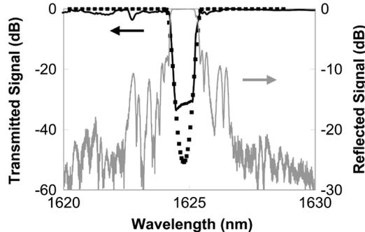
Fig. 2. Transmission (black) and reflection (gray) spectral plots of a grating made with 1000- $\mu\text{J}/\text{pulse}$  IR radiation. The simulation of a 6.4-mm-long grating with a Gaussian profile and  $\Delta n = 1.5 \times 10^{-3}$  is superposed on the measured transmission plot (dotted line).
