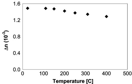
Fig. 5. Annealing behavior of the refractive index modulation in a phosphate glass Bragg grating.
