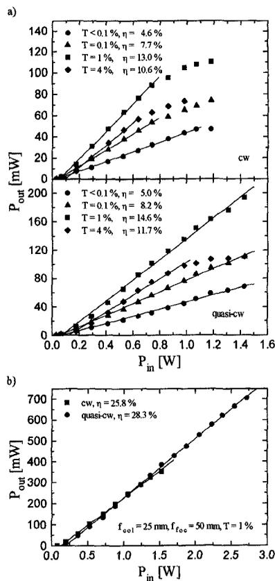
**CTuM71 Fig. 1.** Laser characteristics of the 2-mm-long Yb( $4 \cdot 10^{21} \text{cm}^{-3}$ ), Er( $5 \cdot 10^{19} \text{cm}^{-3}$ ); glass in the cw and quasi-cw mode when pumping with a) the polarization-coupled laser diodes ( $f = 3$  cm) and b) the pigtail laser diode.
