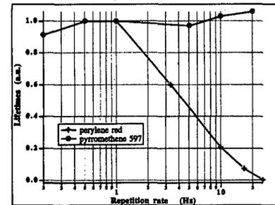
CTh15 Fig. 3 Relative lifetimes versus repetition rate of perylene and pyromethene xerogel doped samples used as gain media in solid-state lasers (normalized at one for 1 Hz repetition rate).
