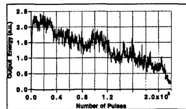
CTh15 Fig. 2 Output energy function of the number of pulses using an oxygen-free pyromethene 597 doped sample (MTEOS matrix, concentration = 5.5 x 10<sup>-4</sup> mol/l, thickness = 1 cm).
