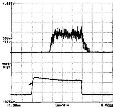
CTh14 Fig. 1 Lamp pump pulse and laser pulse.
