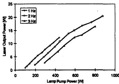
CTh14 Fig. 3 Laser output power vs lamp pump power.
