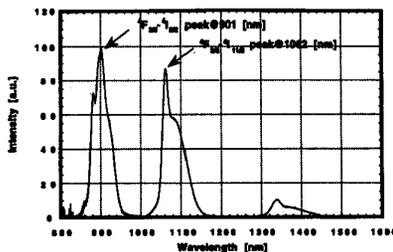
CTH13 Fig. 1 The fluorescence spectrum Nd Zeolite X-doped  $\text{SiO}_2$  ( $\text{Nd}_2\text{O}_3$ :1.0wt%).
