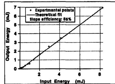
CTh15 Fig. 1 Conversion efficiency of the laser cavity emitting at 568 nm using a pyromethene 580 doped sample (MTEOS matrix, concentration = 2 x 10<sup>-4</sup> mol/l, thickness = 1 cm).
