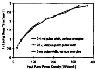
CTh14 Fig. 2 The effect of peak pump power density on the reciprocal of the lasing delay time for a 3 mm x 80 mm rod.
