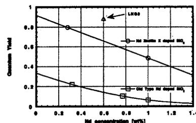
CTH13 Fig. 2 The quantum yield of Nd Zeolite X-doped  $\text{SiO}_2$  and other glasses are shown. Nd Zeolite X-doped  $\text{SiO}_2$  is more improved than the old type Nd-doped  $\text{SiO}_2$ .<sup>6</sup>
