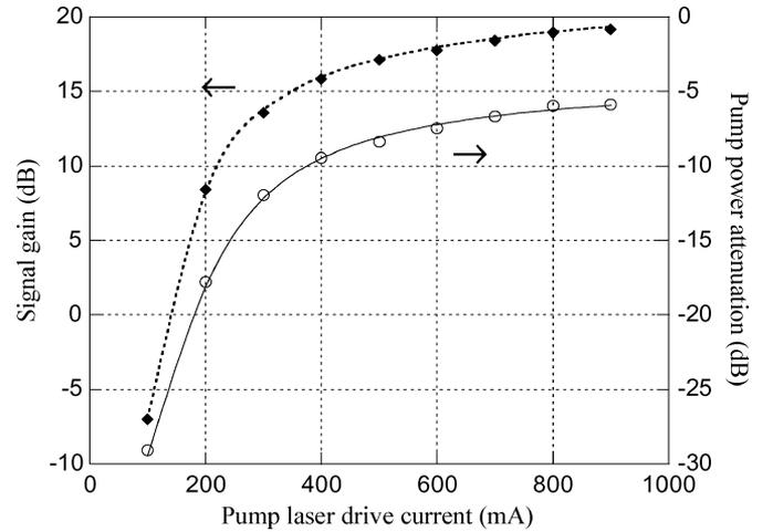
Fig. 3. Measured pump attenuation ( $\circ$ ) and signal gain ( $\blacklozenge$ ) and numerical values (full and broken lines) for the best-fit parameters, as a function of the laser diode drive current.
