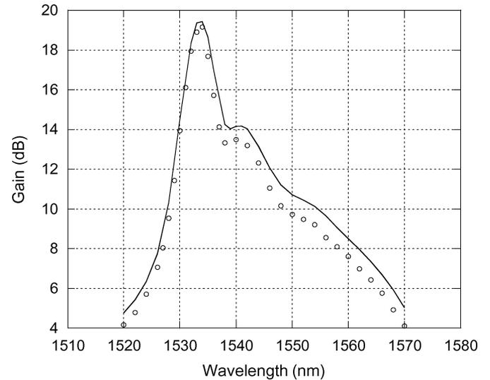
Fig. 8. Measured (o) and numerical (full line) small signal gain spectrum for a laser diode drive current of 900 mA.
