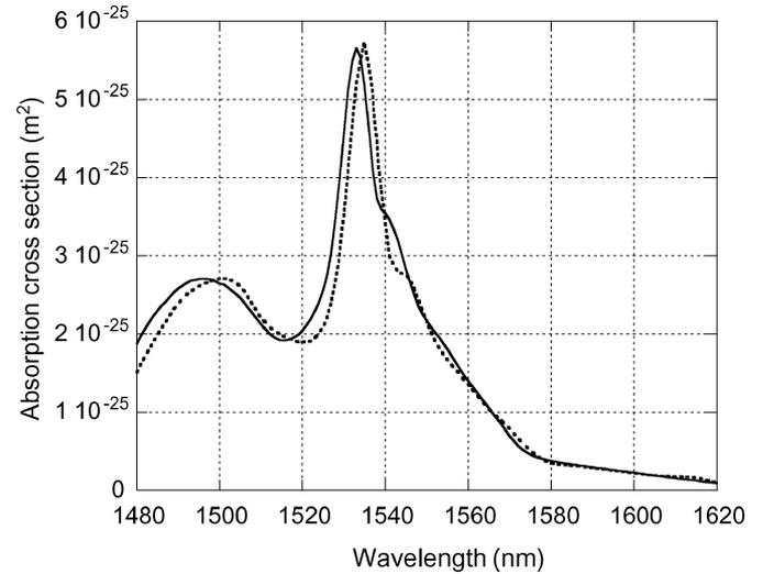
Fig. 7. Initial (broken line) absorption cross section profile (from [18]) and final (full line) profile obtained from the measured ASE<sup>+</sup> power spectrum for a laser diode drive current of 900 mA.
