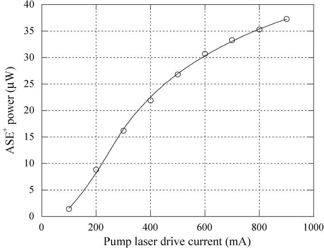
Fig. 4. Measured total ASE<sup>+</sup> power (o) and numerical (full line) values for the best-fit parameters, as a function of the laser diode drive current.
