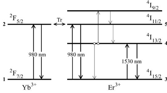
Fig. 1. Energy level scheme of the  $\text{Yb}^{3+}$  –  $\text{Er}^{3+}$ -codoped system in a phosphate glass.
