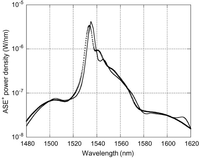
Fig. 5. Measured (o) and numerical (full line) ASE<sup>+</sup> power spectrum, for a laser diode drive current of 900 mA ( $\approx 356$  mW of input pump power).
