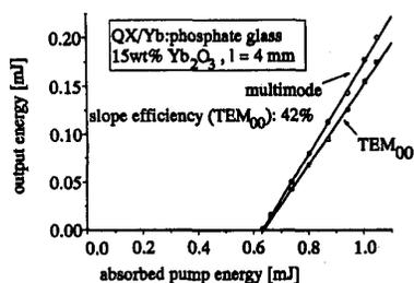
CTH11 Fig. 2 Output versus input characteristics of the transversely diode-pumped Yb:phosphate glass laser.
