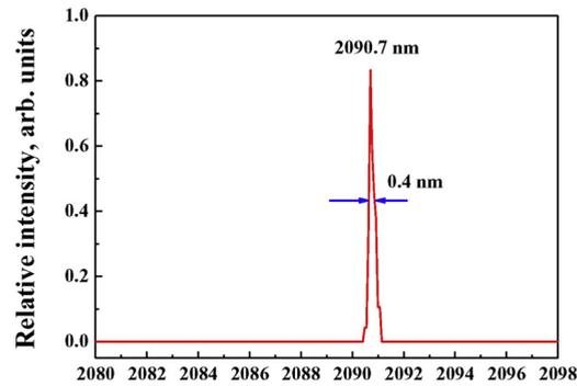
Fig. 5. The output spectrum of the Ho:YAG laser.
