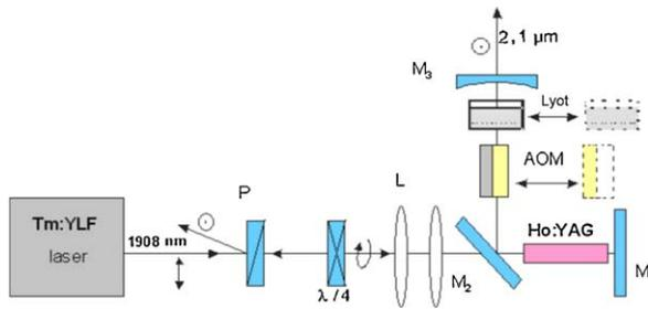
**Fig. 2.** The schematic set-up of the Ho:YAG laser pumped by the Tm:YLF laser with P as a polarizer,  $\lambda/4$  is a quarter wavelength plate, M is the mirror, L is a lens, AOM is the acousto-optical modulator and Lyot is the filter [12].
