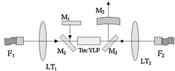
**Fig. 1.** Schematic set-up of the Tm:YLF laser.  $F_1$  and  $F_2$  are fiber outputs of the fiber-coupled diode lasers,  $LT_1$  and  $LT_2$  are lensed telescopes,  $M_1$  is the high-reflection mirror,  $M_2$  are transparent mirrors for the pumping beam and reflective mirrors for the generation beam, and  $M_3$  is the output coupler [10].
