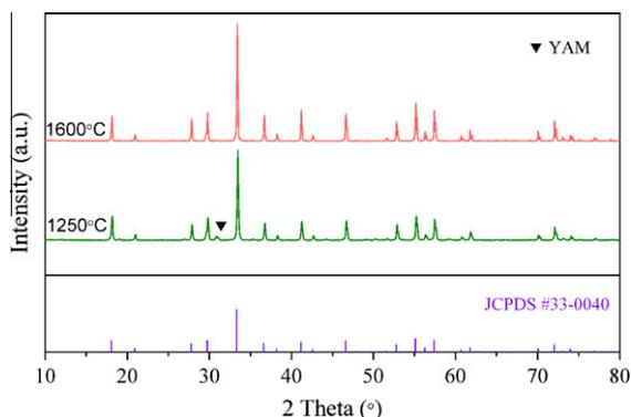
Fig. 2. XRD patterns of the powder compacts sintered at different temperatures for 6 h.
