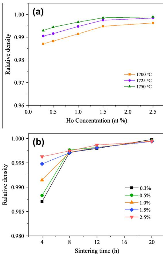
Fig. 3. Relative density of Ho:YAG specimens (a) as a function of sintering temperature and (b) as a function of sintering time.
