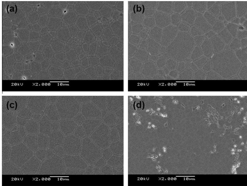
**Fig. 4.** SEM morphologies of 1.0 at.% Ho:YAG sintered at (a) 1650 °C; (b) 1700 °C; (c) 1750 °C and (d) 1780 °C for 8 h.
