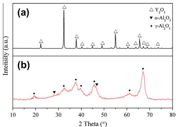
Fig. 1. XRD patterns for the starting materials (a)  $\text{Y}_2\text{O}_3$  and (b)  $\text{Al}_2\text{O}_3$ .
