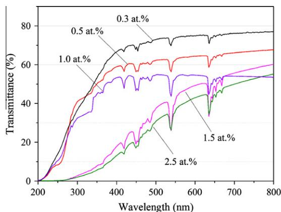
Fig. 6. Optical transmittance of Ho:YAG ceramics sintered at 1700 °C for 4 h with different Ho concentration.
