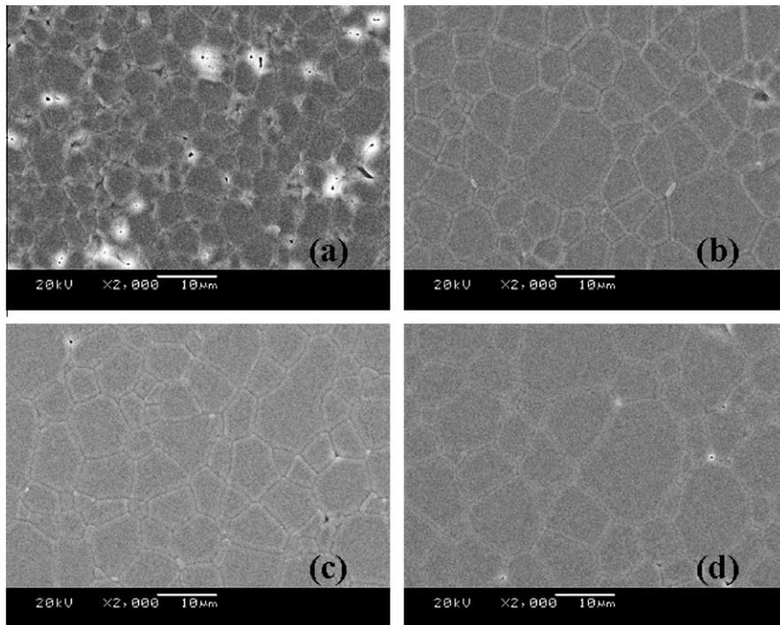
**Fig. 5.** The microstructures of 1.0 at.% Ho:YAG ceramics sintered at 1700 °C for (a) 1 h; (b) 4 h; (c) 8 h and (d) 12 h under vacuum.
