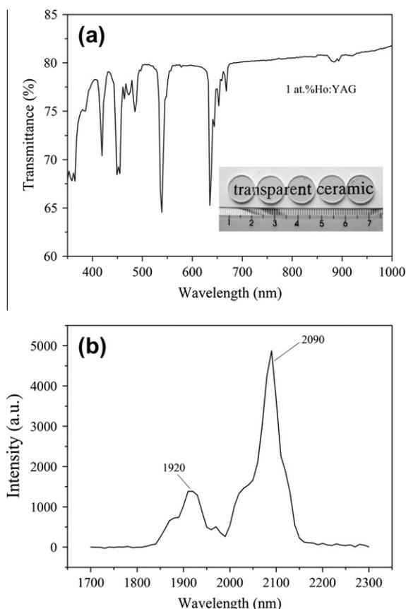
Fig. 7. (a) In-line transmission spectrum of 1.0 at.% Ho:YAG ceramics (2 mm thick) sintered at 1700 °C for 12 h. Inset is a photo showing the appearances of transparent Ho:YAG specimens; and (b) fluorescence spectra of the prepared 1.0 at.% Ho:YAG ceramic.
